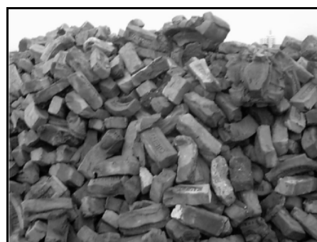
Fig. 1 Over Burnt Bricks
