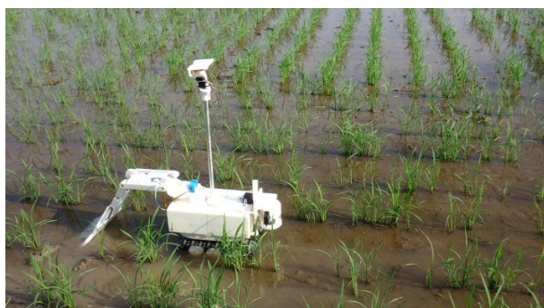
Fig. 11 Experiment of the posture control in paddy field
