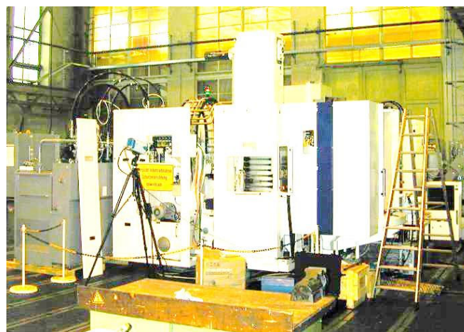
Fig. 2 Machining centre and thermography camera in factory work floor
