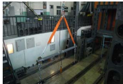
Fig. 7 Load test of single-beam hoist
