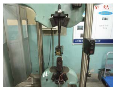
Fig. 6 Load test of the releasing device
