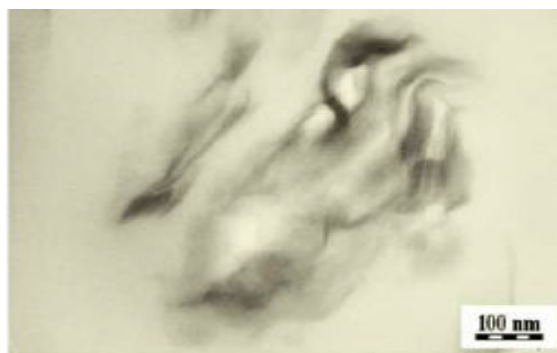
Fig. 4 TEM analysis of composition: Dellite 67G in PP matrix
