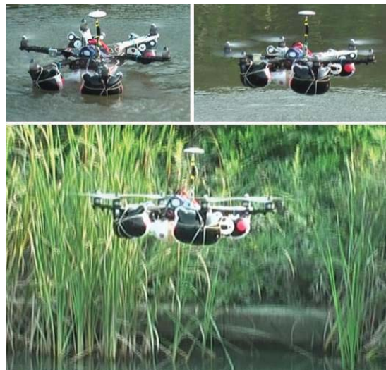
Fig. 10 Successful test of taking off of hexarotor from the water
