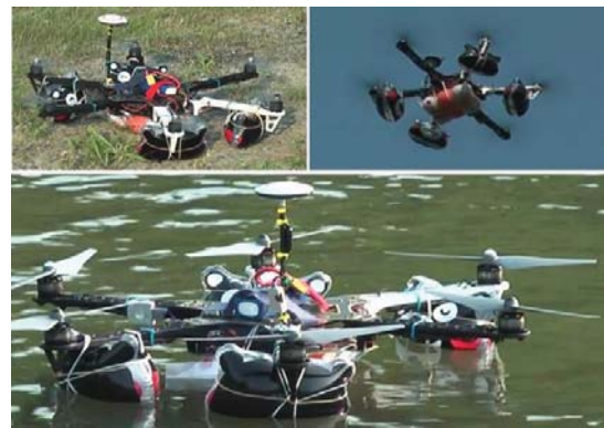
Fig. 9 Successful test of the floating hexarotor with the air balloons and landing on the water
