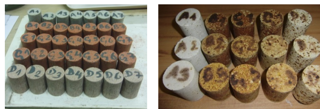
Fig. 3 Specimens before and after firing, fire 1, 2, 3
