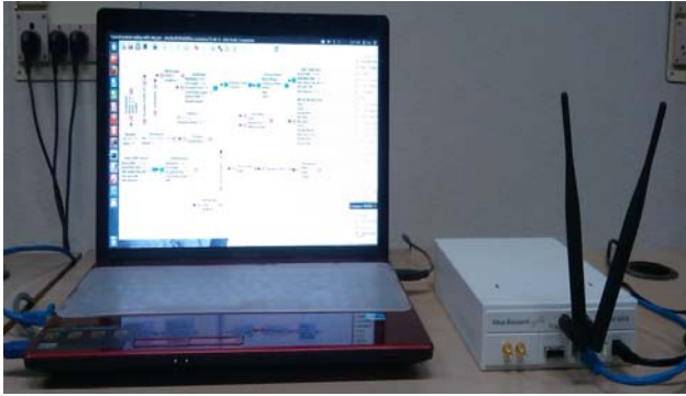
Fig. 3 Software Defined Radio development test bed
