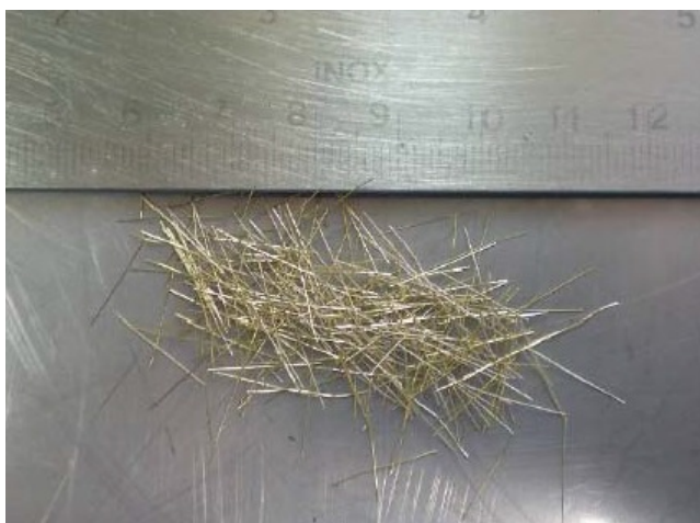
Fig. 1 Fibers (carbon steel coated brass) used in the experiment
