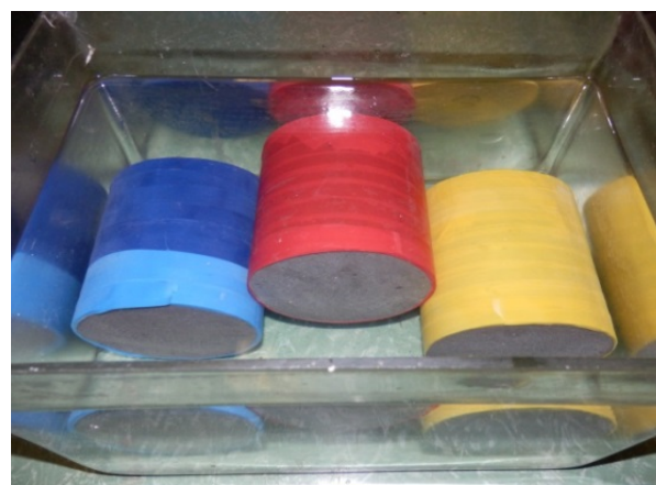
Fig. 2 Samples immersed in the 3% NaCl
