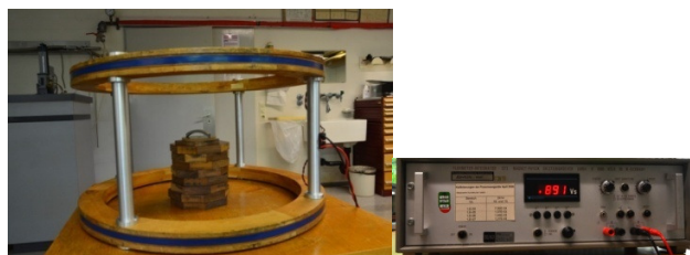
Fig. 2 A Helmholtz coils with magnet (left) and flux meter (right)
