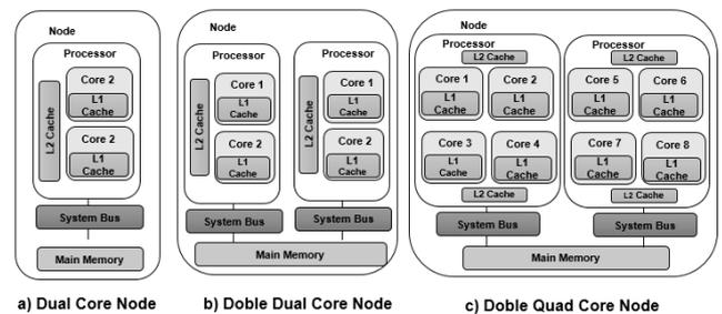
Fig. 6 Different Multicore Architecture
