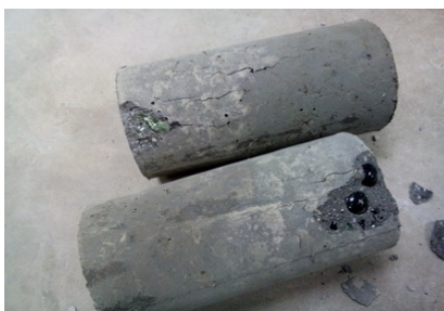
Fig. 4 Crack pattern in Concrete cylinder
