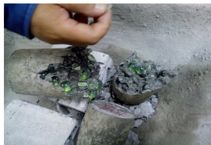
Fig. 5 Internal bond in Concrete cylinder
