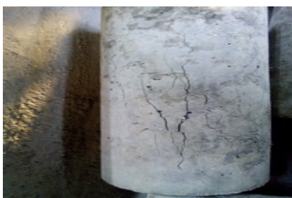
Fig. 3 Crack pattern in Concrete cylinder
