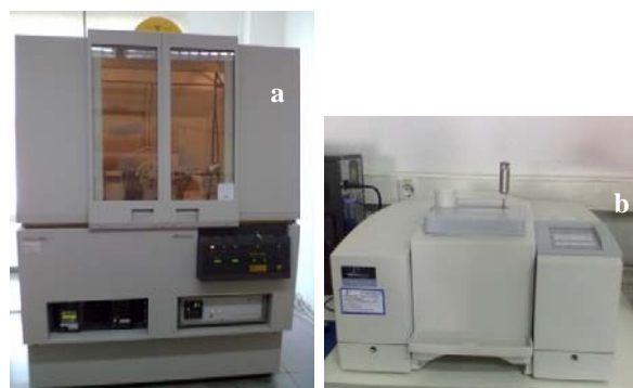
Fig. 2 (a) Philips PANalytical XPert Pro XRD, (b) Perkin Elmer Spectrum One FT-IR Spectroscopy
