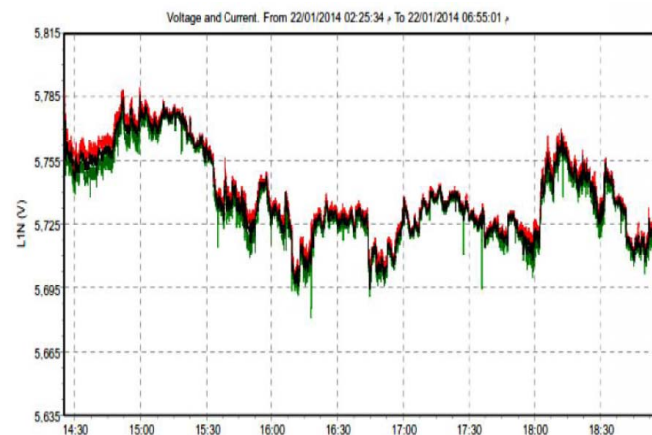
Fig. 4 Voltage variation in Al-Nasim Dairy
