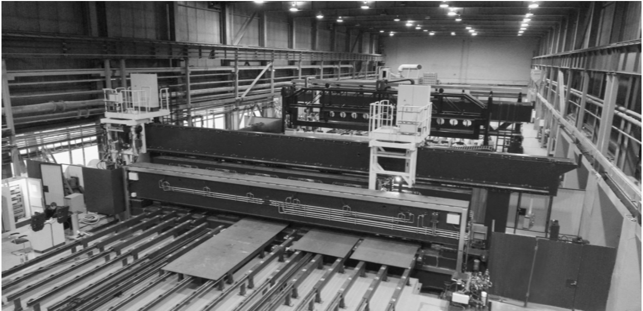
Fig. 7 Sample of flat panel production line
