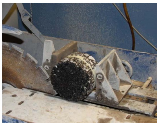
Fig. 2 Cutting a sample using a laboratory saw
