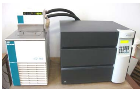
Fig. 3 Apparatus Holometrix 2300 for determination of thermal conductivity
