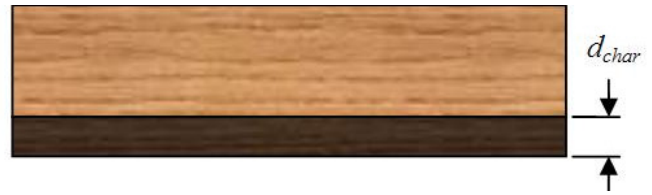
Fig. 2 Charring of timber – one dimensional
