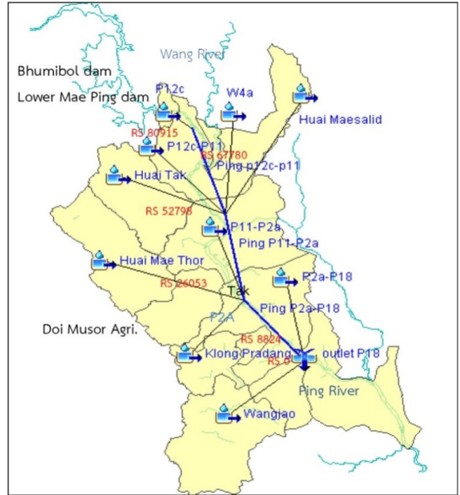
Fig. 3 Schematic map and location of lateral inflow from all catchments of the Ping River used in the HEC-HMS model
