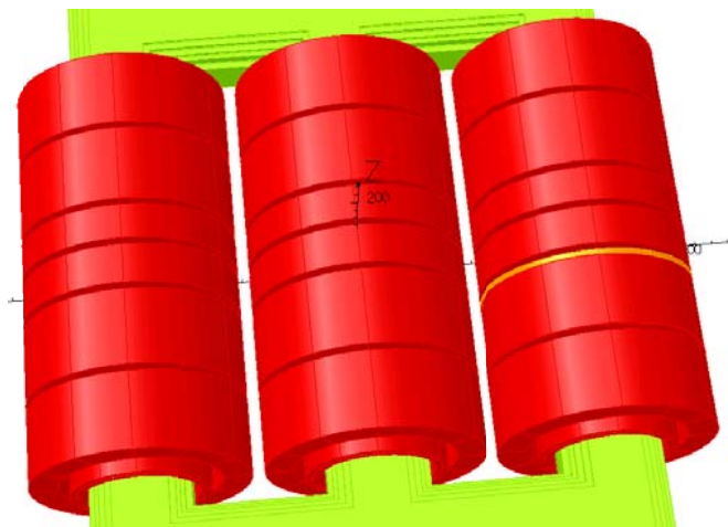
Fig. 8 Model of the faulty transformer TO294-22kV with axial short circuit (orange)
