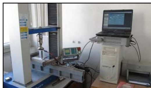
Fig. 2 Evaluation of electrical properties under loading
