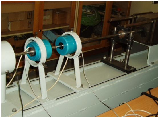
Fig. 2 The Split Hopkinson Pressure Bar
