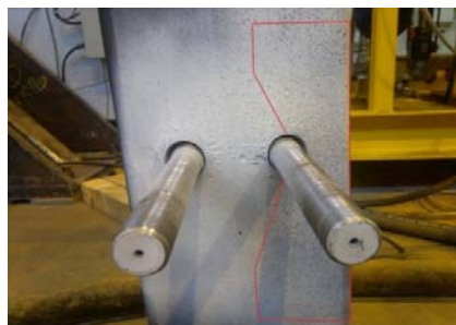
Fig. 7 Area captured by DIC system
