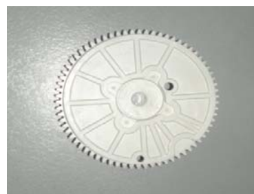
Fig. 2 (a) Plastic, 70 teeth, 3.5cm diameter gear
