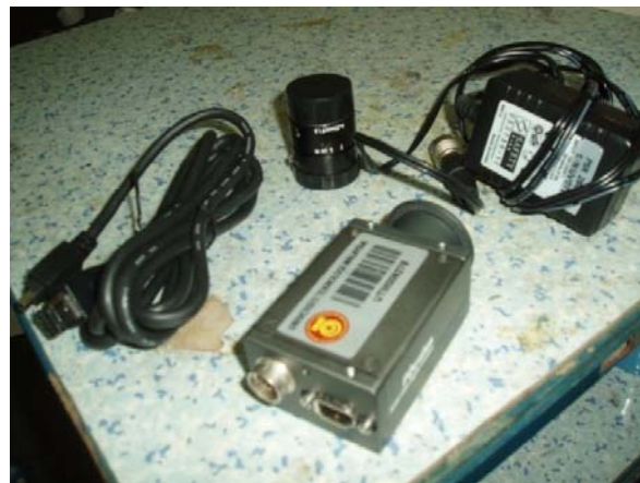
Fig. 4 Progressive Scan Monochrome Camera for the current study
