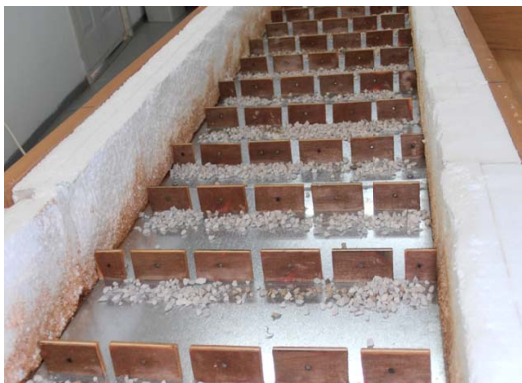
Fig. 8 Self-cleaning channel in percentage of the sediment (Taken from upstream perspective)
