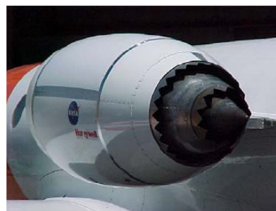
Fig. 1 Chevron nozzle flight test with Honeywell's Falcon 20 test plane: A close-up view of engine and nozzle (Adopted from [2])
