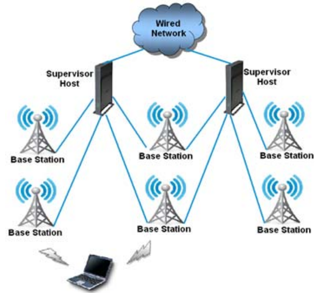
Fig. 3 Underlying architecture of M-TCP
