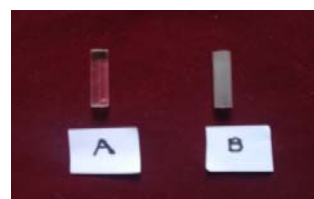
Fig. 1 Samples SBN1 (A: Before Annealing, B: After Annealing)
