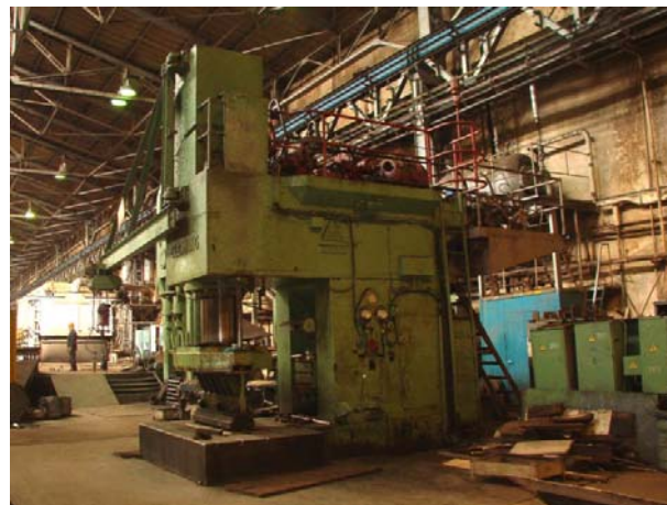
Fig. 1 Press "Clearing", 3500 kN (350t) capacity
