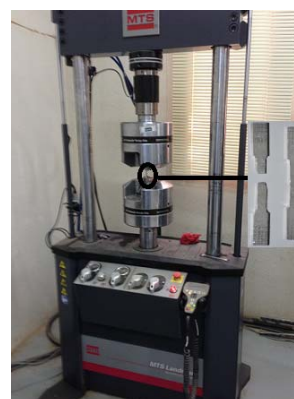
Fig. 2 Commercial pure aluminum sample during tensile test
