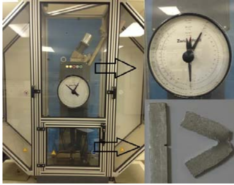
Fig. 3 Impact test machine using in this research
