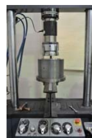
Fig. 1 ECAP die set-up used in this research
