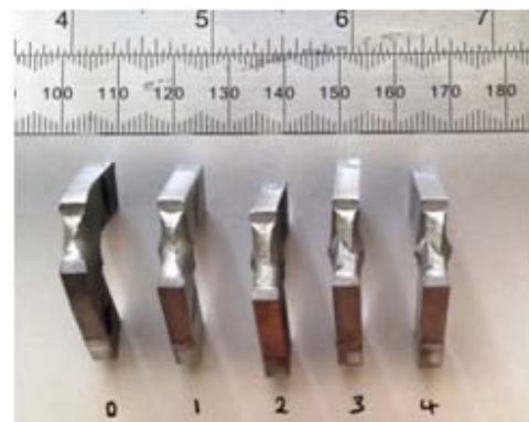
Fig. 11 Fracture surfaces of commercial pure Al before and after ECAP process as a function of pass numbers
