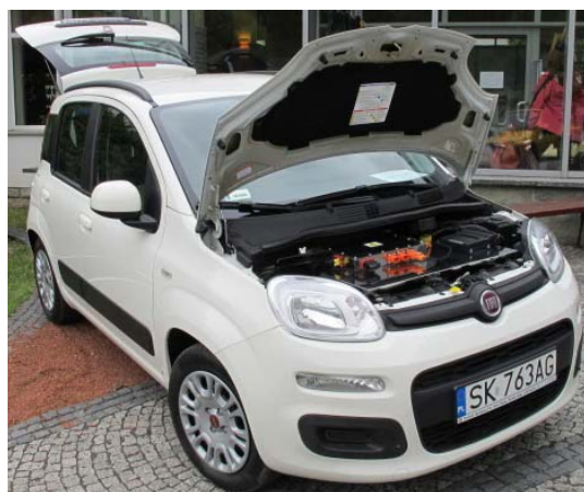
Fig. 2 Fiat Panda with Komel's traction motor – research and development project no. NR01-0084-10
