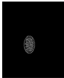
Fig. 9 Edge Detection using Canny Algorithm
