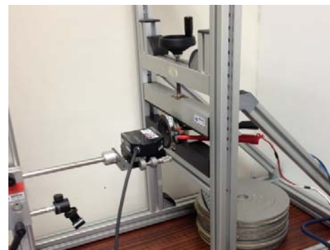
Fig. 2 A two-inch MCL placed on the fixture of the Klippel analyzer system.
