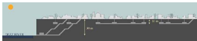
Fig. 3 The level of Shavadan and Dez River in Dezful
