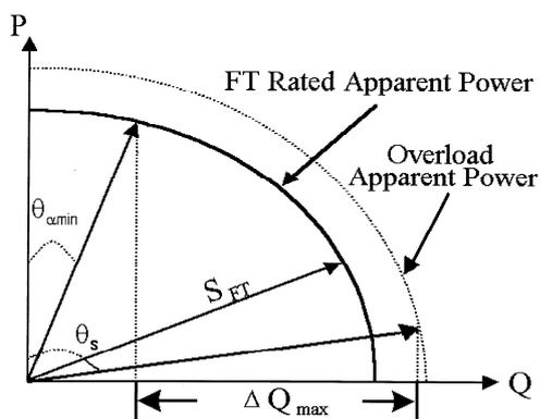
Fig. 1 The load curves of the dc EAF
