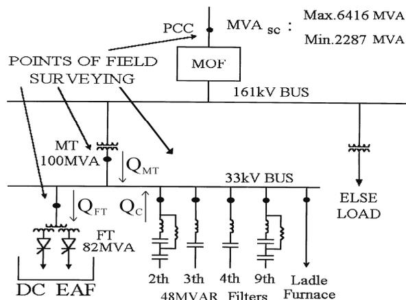
Fig. 2 Single-line diagram of steel factory A
