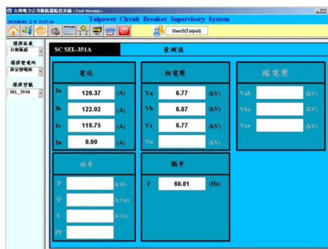
Fig. 9 The display of SEL-351A parameters measurement result
