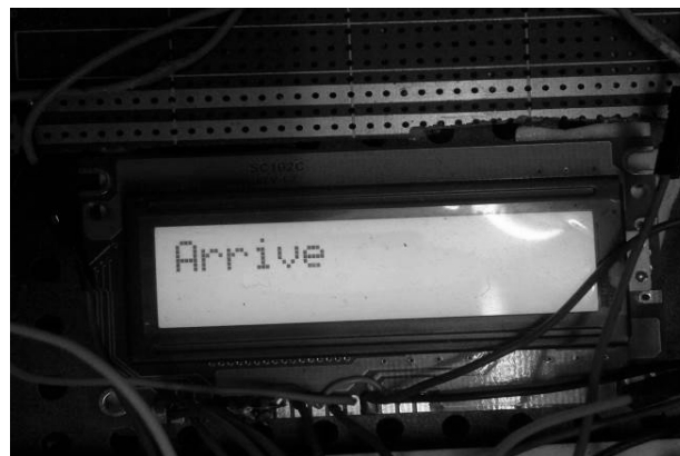
Fig. 16 Station arrival indication
