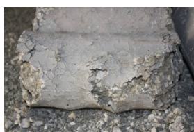
Fig. 6 Decomposition of a specimen exposed to 900°C
