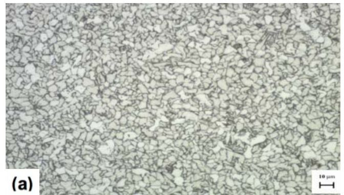
Fig. 5 TMAZ of (a) underwater FSW plate and (b) air FSW plate
