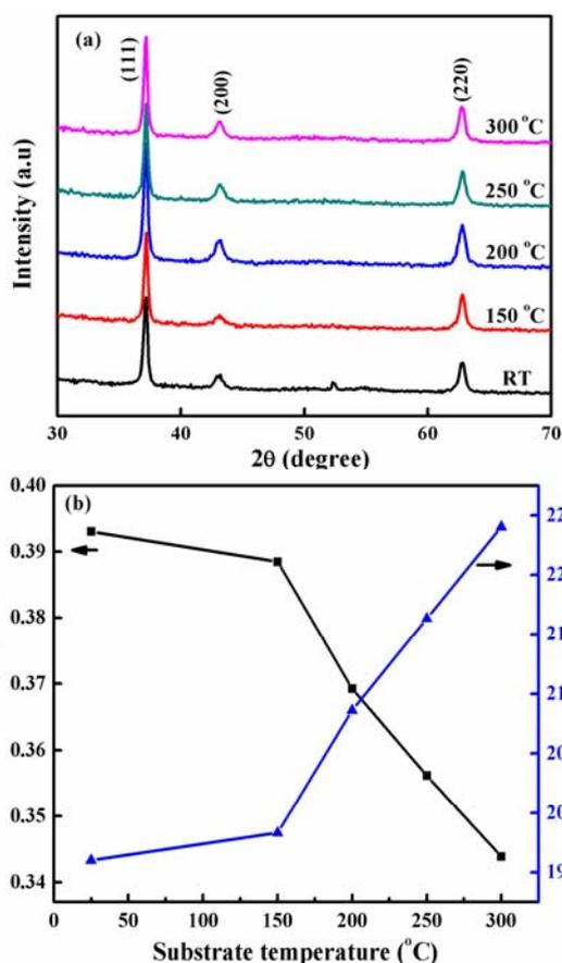
Fig. 1 (a) X-ray diffraction  $\theta$ - $2\theta$  scan data and (b) FWHM and grain size of NiO (111) diffraction peak for p-Ni<sub>1-x</sub>O:Li thin films prepared at various substrate temperatures
