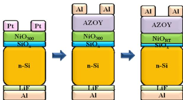
Fig. 5 Improvement structures of p-Ni<sub>1-x</sub>O:Li/n-Si HJSC
