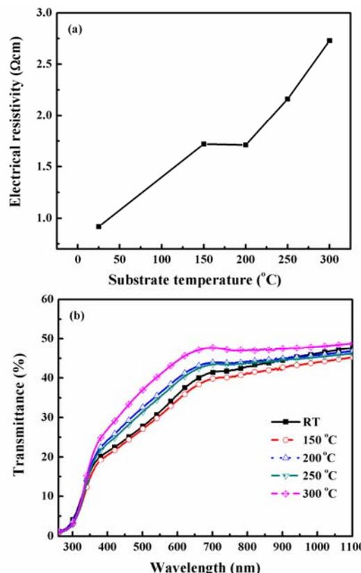
Fig. 2 (a) Electrical resistivity and (b) optical transmittance spectra of p-Ni<sub>1-x</sub>O: Li thin films (with glass substrate) deposited at various substrate temperatures
