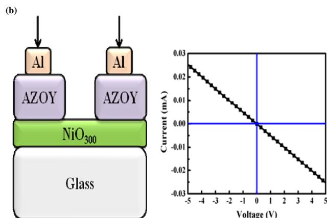
Fig. 3 (a)  $J$ - $V$  characteristics of cells measured under  $100 \text{ mW}/\text{cm}^2$  illumination (AM1.5 condition) for Pt/ $\text{NiO}_{300}$ /n-Si, Al/AZOY/ $\text{NiO}_{300}$ /n-Si, Al/AZOY/ $\text{NiO}_{\text{RT}}$ /n-Si, respectively. (b)  $I$ - $V$  characteristics of Al/AZOY/ $\text{NiO}_{300}$  HJ
