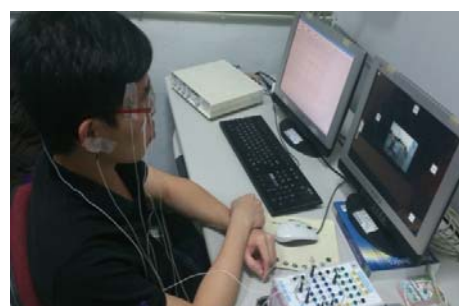
Fig. 3 User operating environment for robot control by brain waves
