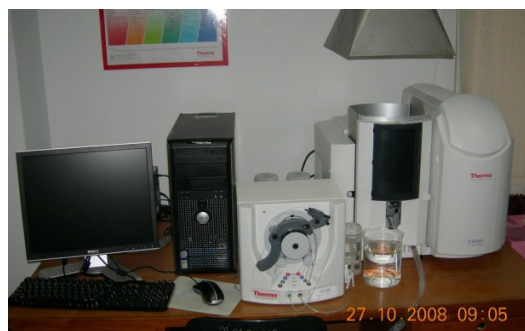
Fig. 4 Atomic Absorption Spectrophotometer Instrument (THERMO series)
