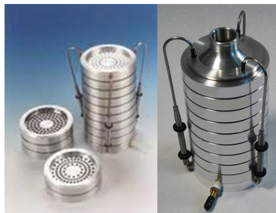
Fig. 3 Eight Stage non- Aiable Cascade Impactor
