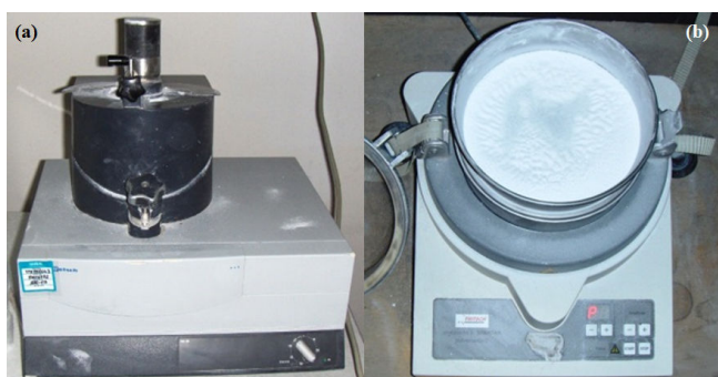
Fig. 1 (a) Grinding process, (b) Sieving process
