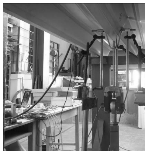
Fig. 4 Measuring instruments to vertical deflection
