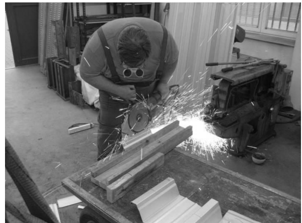
Fig. 7 Preparation the test specimen
