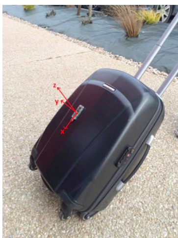
Fig. 4 Slam Stick USB Key on the Luggage
