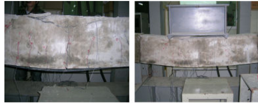
Fig. 13 Bonded FRP failure mode
