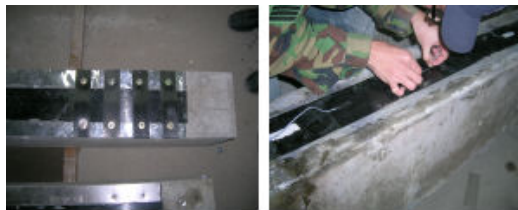
Fig. 6 Intermediate laminates and LVDT setup
