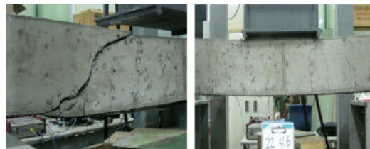
Fig. 15 Anchored titanium strengthened RC structure failure mode
