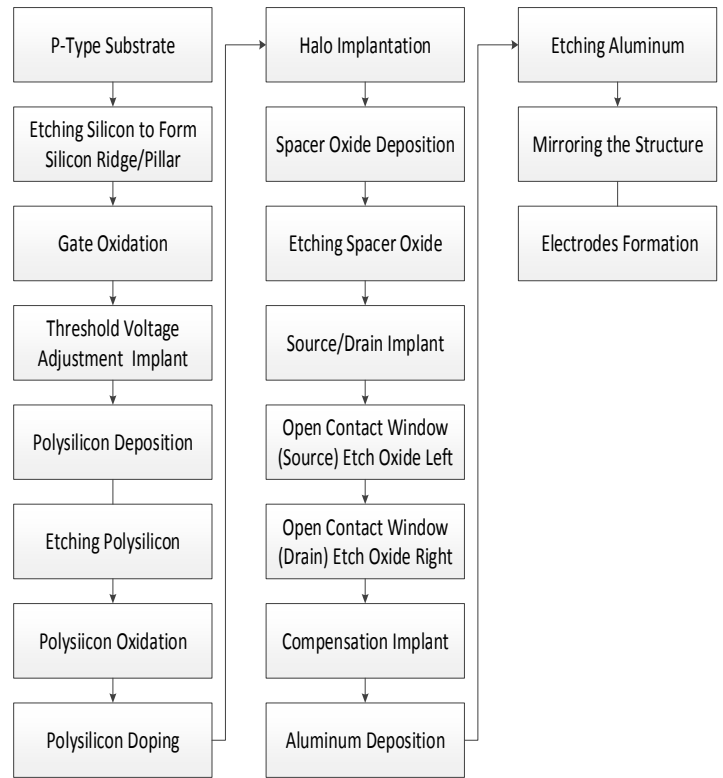
Fig. 2 Vertical DG-MOSFET's Process Simulation Flowchart
