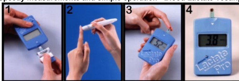
1 Insert the test strip into the strip inlet of the meter. 2 Collection of the blood. 3 Blood is automatically aspirated and measurement begins. 4 The measurement result is displayed in 60 seconds
