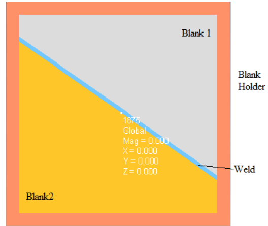
Fig. 3 Different zones of the blank under consideration
